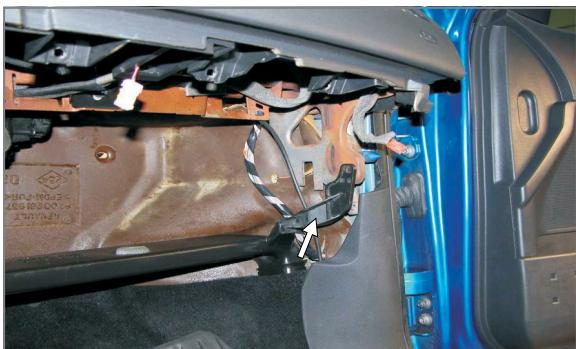
**EN** Remove the protecting device
