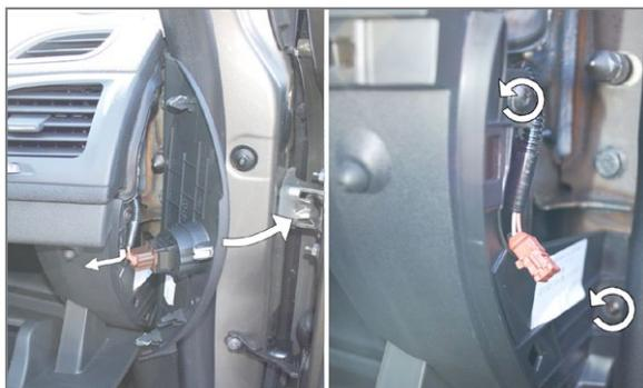
(EN) Remove the upholstery panel. Disconnect the electric circuit. Loosen the screws and remove the upper wall of the locker
