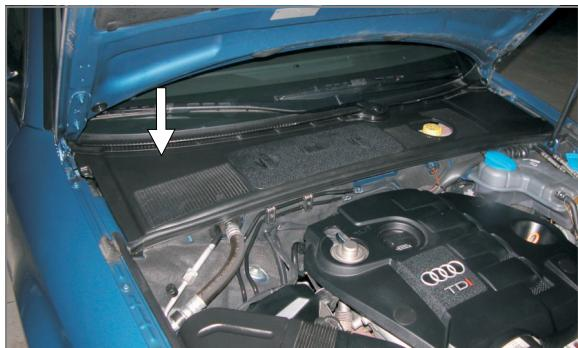
Pollen filter is located behind the engine chamber.
