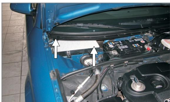
Gently remove the old filter, put in the new one and carry out the opposite to all the previously mentioned operations in the reversed order
