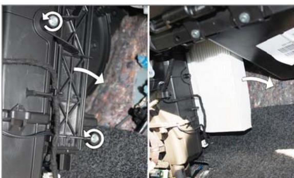
**(EN)** Loosen the screws and remove the cover of the filter. Gently remove the old filter, put in the new one and carry out the opposite to all the previously mentioned operations in the reversed order
