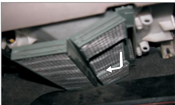
(EN) Remove the old filter, insert the new one and carry out the opposite to all the previous operation at the reversed order
