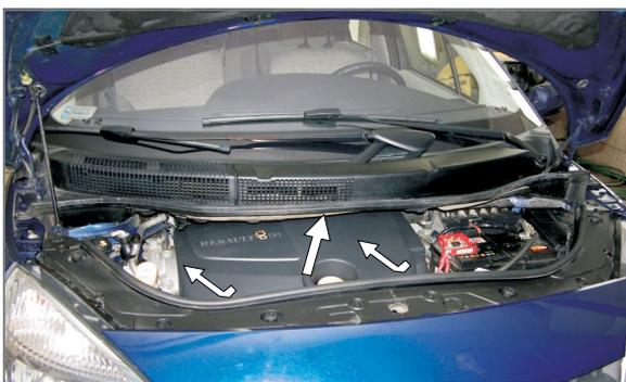
EN Remove the engine housing
