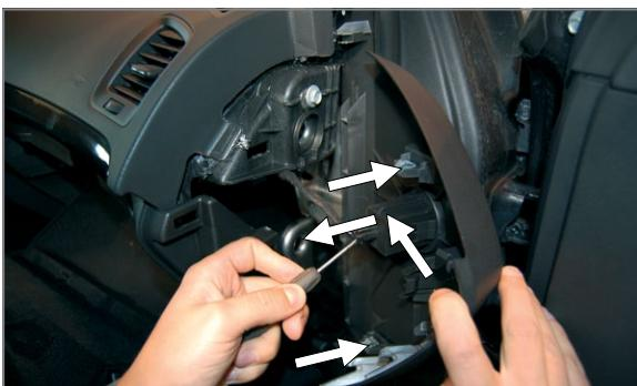
**EN** Remove the screen segment. Disconnect the electric circuit
