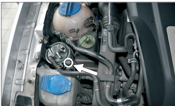
(EN) Loosen the filter clamping ring screws, remove used filter
