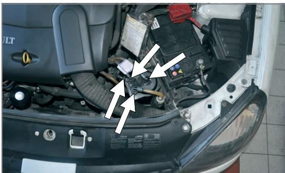
(EN) Disconnect pipes clamp connectors on diesel oil filter
