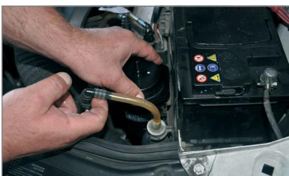
(EN) Connect the cables to new filter
