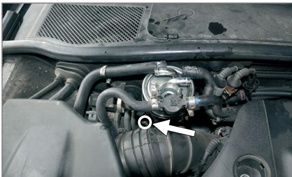
**EN** Place filter in the seat and fasten filter clamping ring
