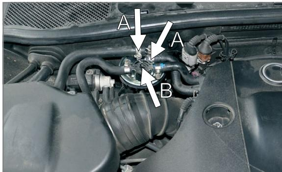
**EN** Fix fuel hoses (A), regulation valve and clamp fastening the valve (B).
