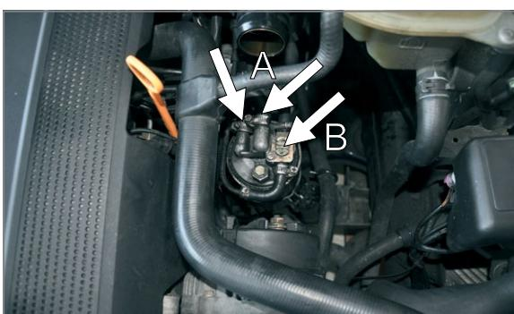
(EN) Loosen bands, take hoses off (A) and regulating valve (B), off fuel filter head
