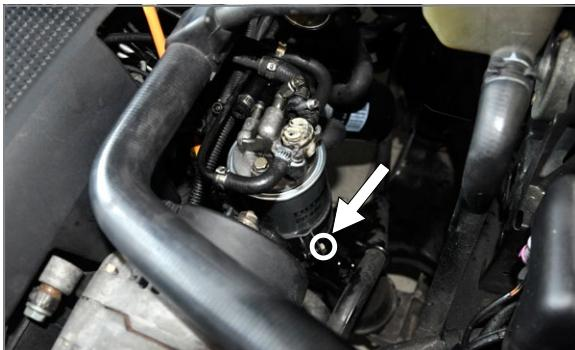
**EN** Install filter in seat, fasten clamping ring screw
