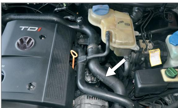
**EN** Fix air intake manifold to the engine, start the engine, check for leakage
