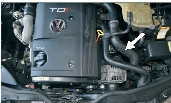
(EN) Remove air intake manifold
