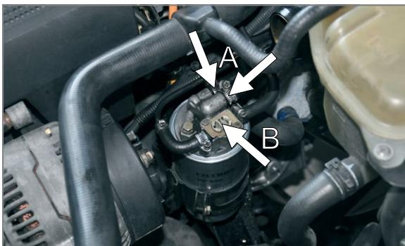
**EN** Install hoses (A) and pressure regulator (B)
