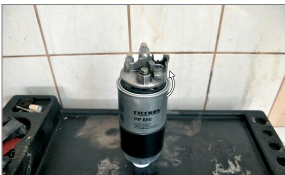
**EN** Remove filter head, fill new filter with clean diesel oil, fix filter head
