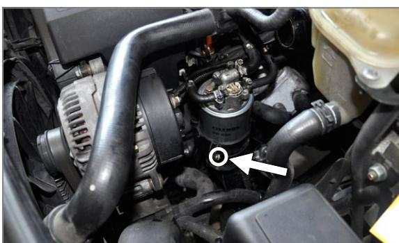
(EN) Loosen clamping ring and take filter out
