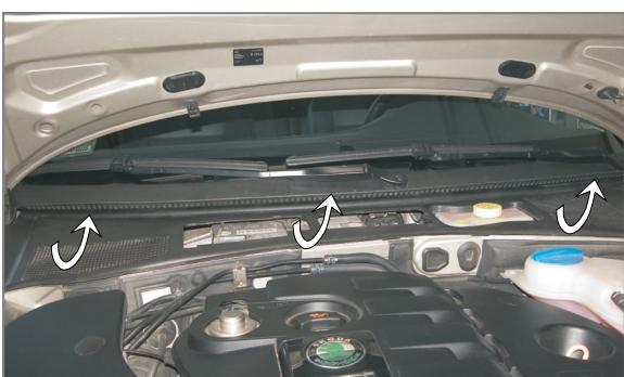
**EN** Remove the screen under the windshield by turning it as shown in the picture
