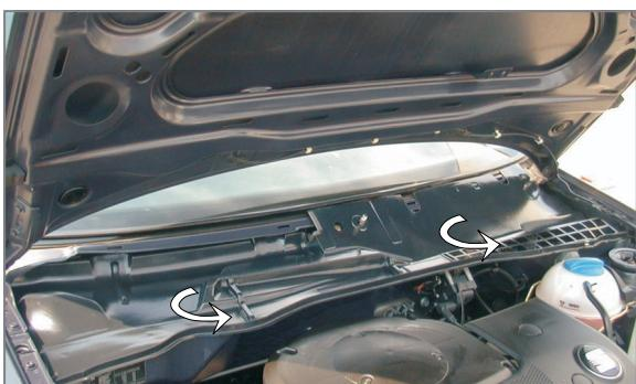
EN Remove the filter housing
