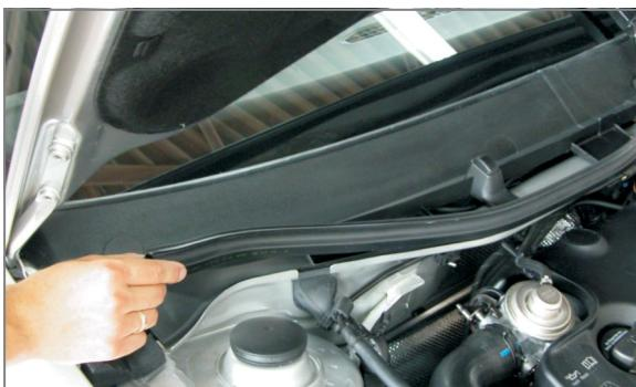
**EN** Remove the rubber seal
