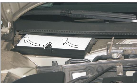
**EN** Remove the filter lock. Remove the old filter from the seat, put the new one in and perform the opposite to all the previous actions in the reverse order
