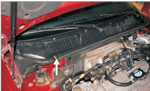
**EN** Remove the rubber seal
