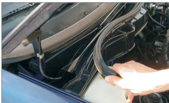
(EN) Remove the rubber seal
