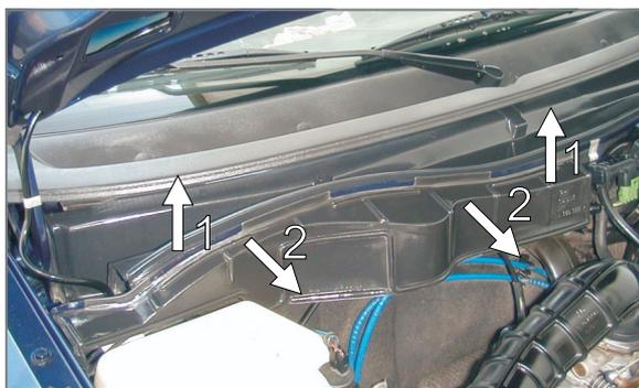
(EN) Remove the electric circuit housing
