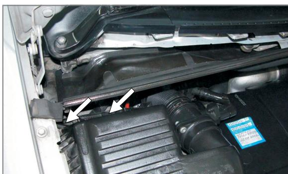
EN Remove the rubber seal
