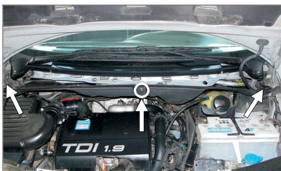
EN Loosen the screws, which hold the cover of the filter chamber
