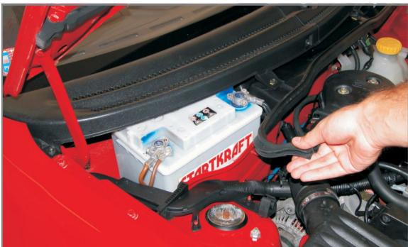
EN Remove the rubber seal
