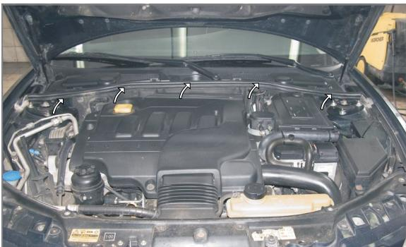
**EN** Remove the rubber seal
