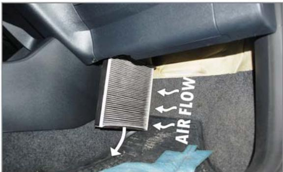
**EN** Unlatch the filter with the frame from its socket. Pollen filter is located behind the engine chamber
