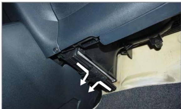
(EN) Move sideways the locks, which hold the cover of the filter chamber
