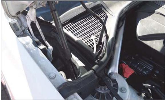
**EN** Remove the rubber seal
