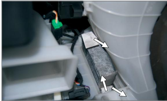
Carefully remove the first filter, the second one will slide downwards.
