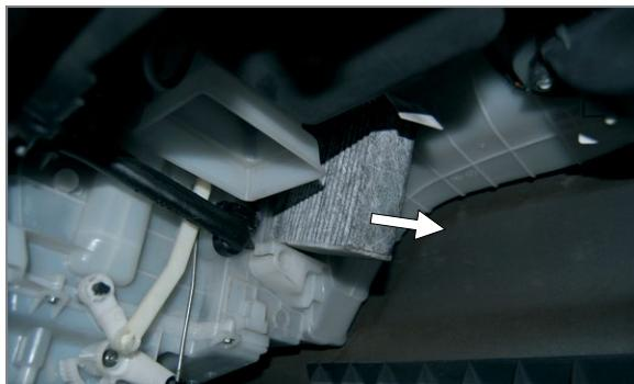
**EN** Open the filter chamber. Carefully remove the first filter, the second one will slide downwards
