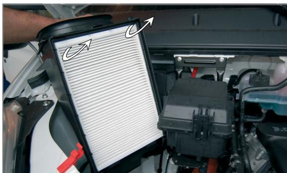
EN Remove the old filter from the seat, put the new one in and perform the opposite to all the previous actions in the reverse order
