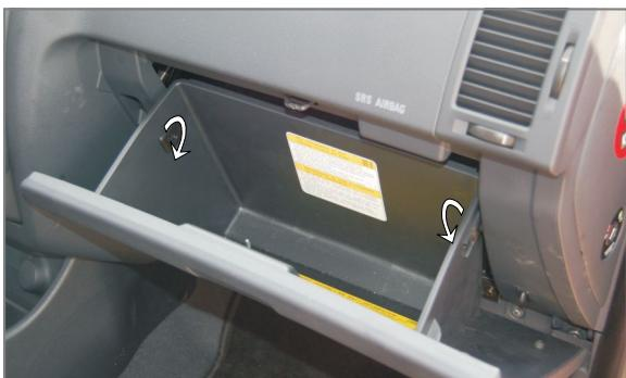
**EN** Remove the glove compartment
