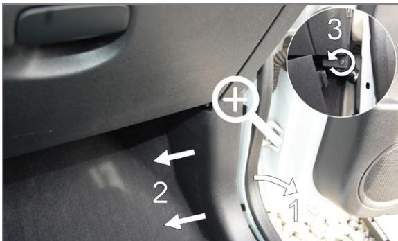
(EN) Remove the rubber seal. Remove the upholstery panel. Loosen the screw
