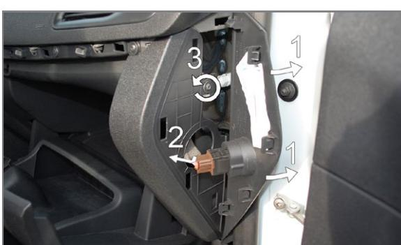
**EN** Remove the upholstery panel. Disconnect the electric circuit. Loosen the screw
