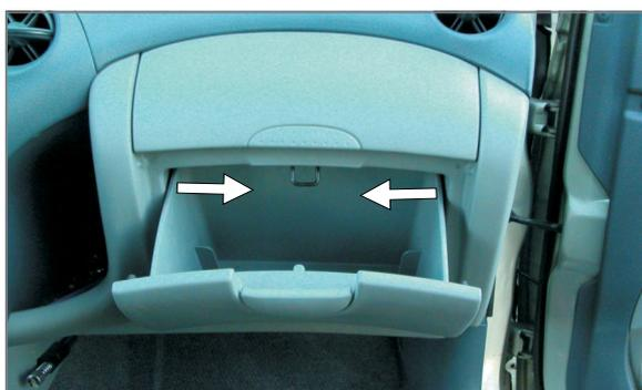
(EN) Open the glove locker, remove the locker
