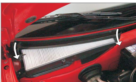
EN Remove the protecting device
