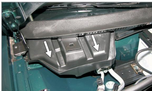
**EN** Remove the filter housing
