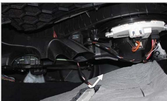
(EN) Disconnect the electric circuit
