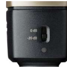
Figure 2: Selector for preattenuation pads
