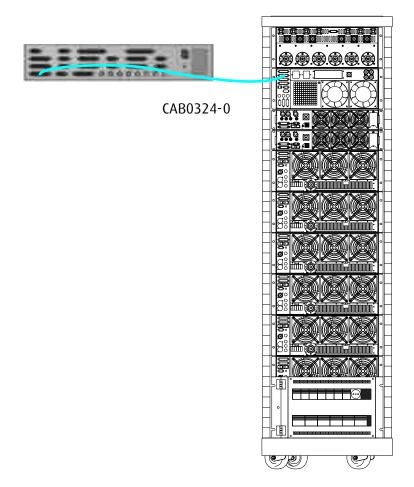
If the equipment is used as a spare, also provide an additional standard extension cable to be inserted into the "PROFILES" connector, DB25, located on the rear panel of the control unit (ELENOS code **CAB0324-0**).
