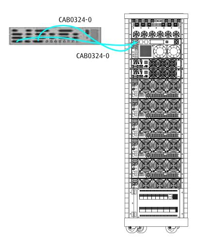
If the system has an audio matrix, this latter cable must be connected the matrix itself and not to the exchange unit.
