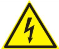
Uninsulated dangerous voltage are inside the enclosure, voltage that may be sufficient to constitute a risk of shock.
