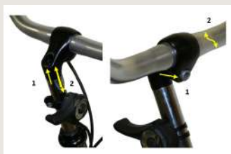
Adjust handlebar height Adjust steering angle
