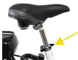
Seat height via quick-release lever
