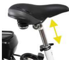
Seat height via quick-release lever
