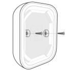
2. Put the siren on the SmartBracket panel and turn it clockwise, then fix the device with a screw.
