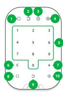
1 - Armed mode indicator 2 - Disarmed mode indicator 3 - Night mode indicator 4 - Malfunction indicator
