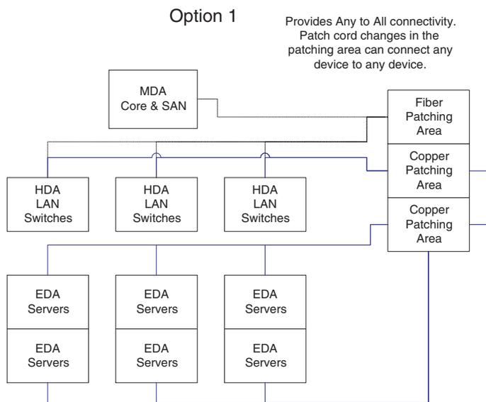
Provides Any to All connectivity. Patch cord changes in the patching area can connect any device to any device.
