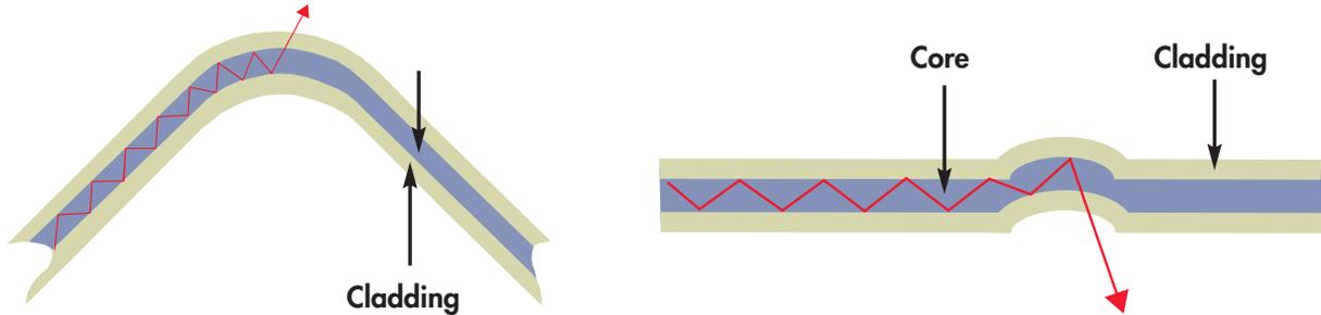
In fiber, the signals and pulses must be understood by the receiver at each end. Running too long a fiber channel can cause errors, as can excessive splices, poor fiber quality and poor installation. Any anomaly that keeps a receiver from registering the pulses will equate to a bit error.
