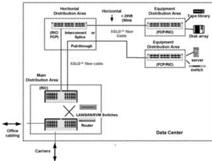
Figure-1: Data Center Centralized Siemon 10G ip™ XGLO Optical Fiber Cabling System Structure
