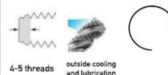
material: HSSE-TiAlN 2B to 1300 N/mm² 41 HRC
