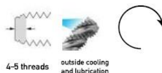
material: HSSE 2B to 900 N/mm² 27.1 HRC
