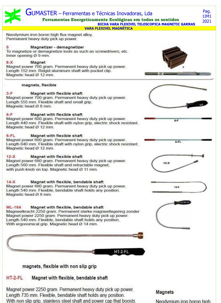
the magnet power to the front of the magnet head, so the magnet
